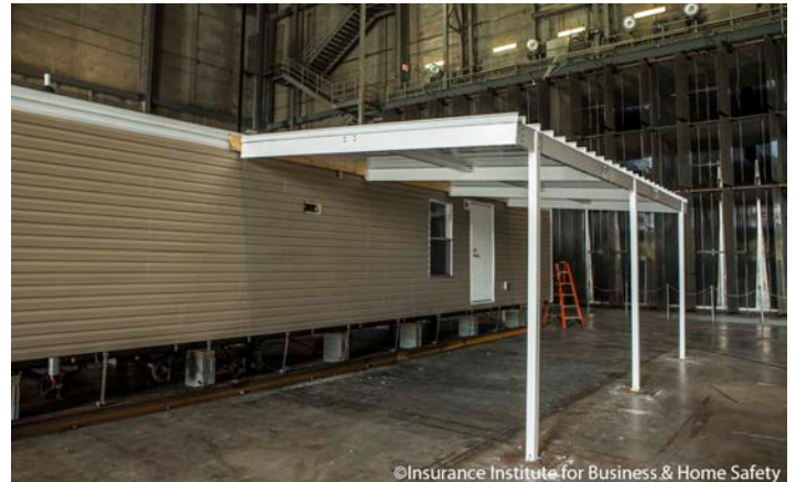
Figure 25. Photo of AAF-based design that withstood wind speeds in excess of 100 mph with no damage. Tests were conducted with both 0.024" and 0.032" thick pans, which were attached to beam between wall and eave using screws with metal/neoprene washers.
