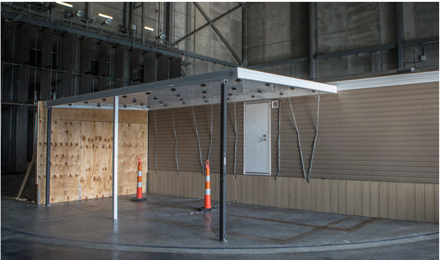
Figure 1. Instrumented carport with skirting and wall blocking wind exit at one end.
