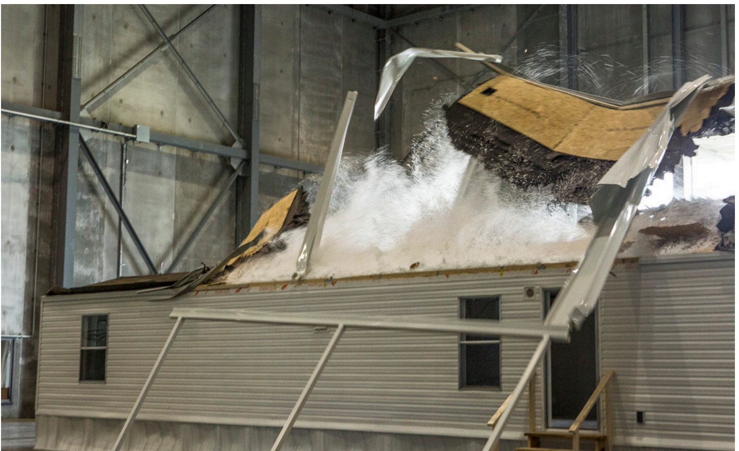
Figure 28. Detaching carport pulled roof sheathing from a manufactured home, introducing blown insulation (white) into the airstream.
