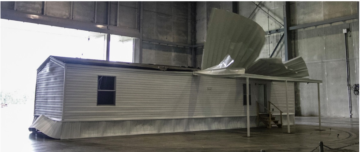
Figure 7. Failure of connections between roof pans and support beam at roof eave.
